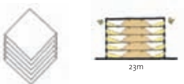
Open plan multi-storey 'big box' requires most intensive artificial lighting and suits only certain uses
