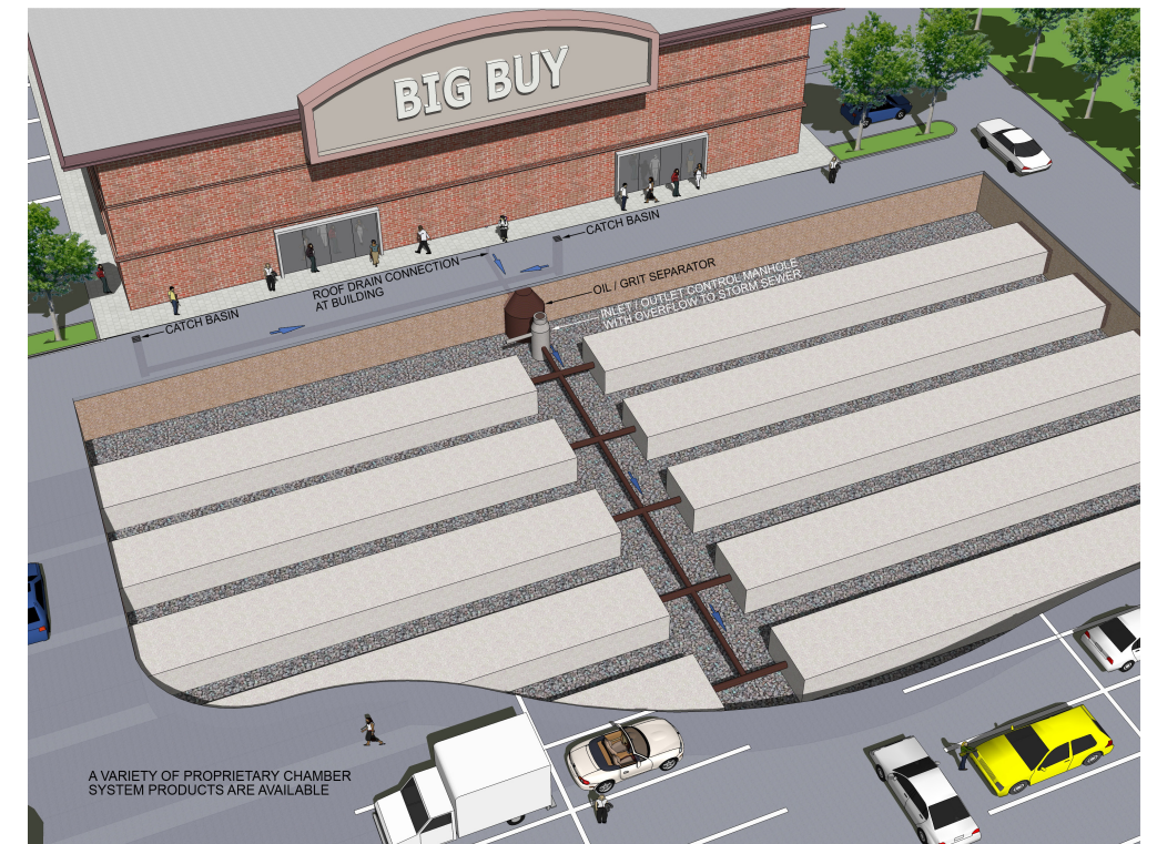
Infiltration Chamber System Under Parking Lot
